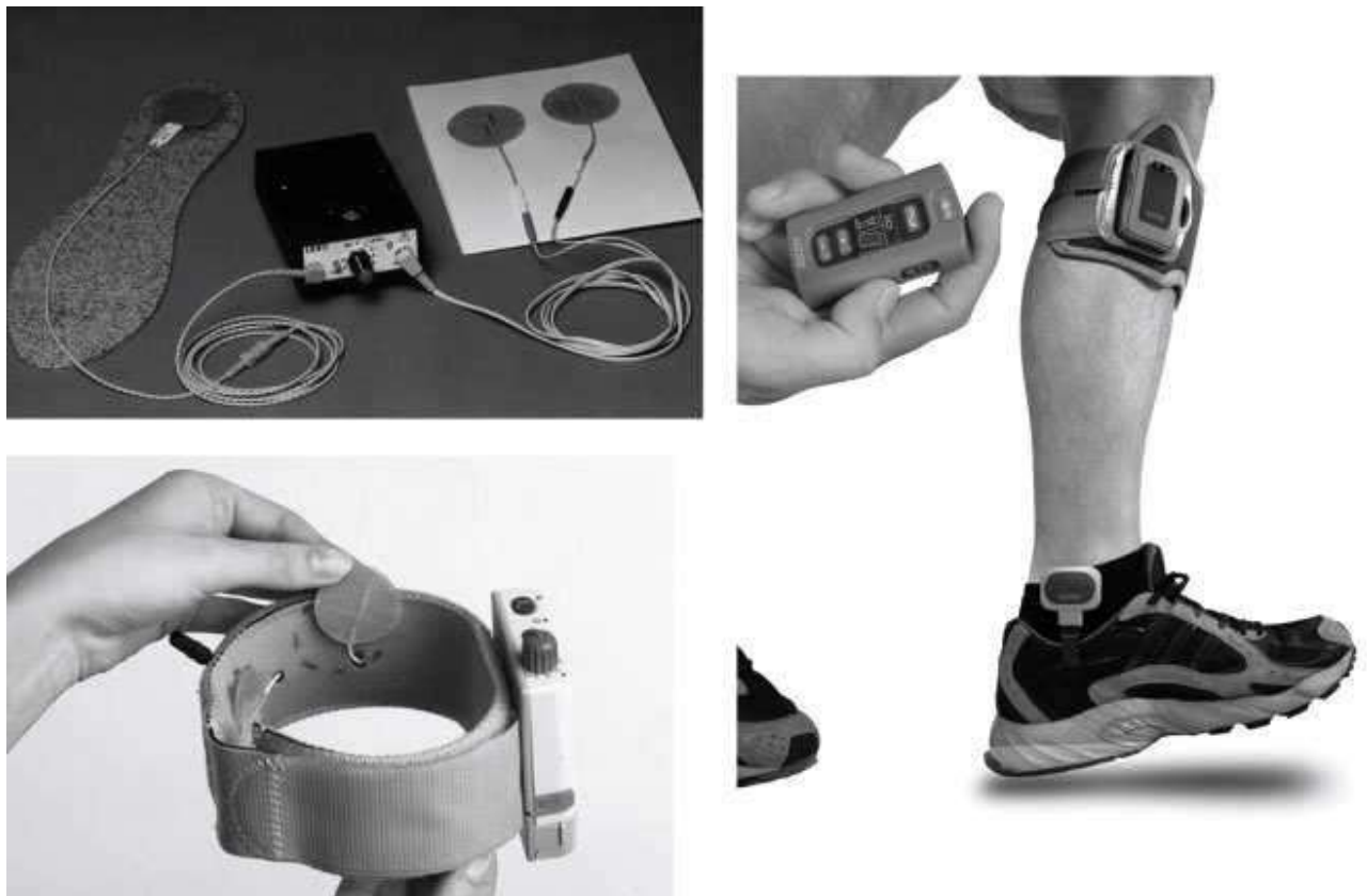
FIGURE 3. Three FDA-approved transcutaneous peroneal nerve stimulators.
