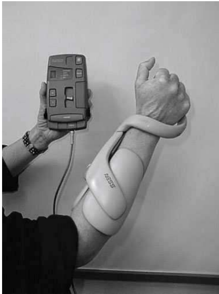
FIGURE 1. A hybrid brace-transcutaneous neuroprosthesis system that is worn on the hand and forearm.
