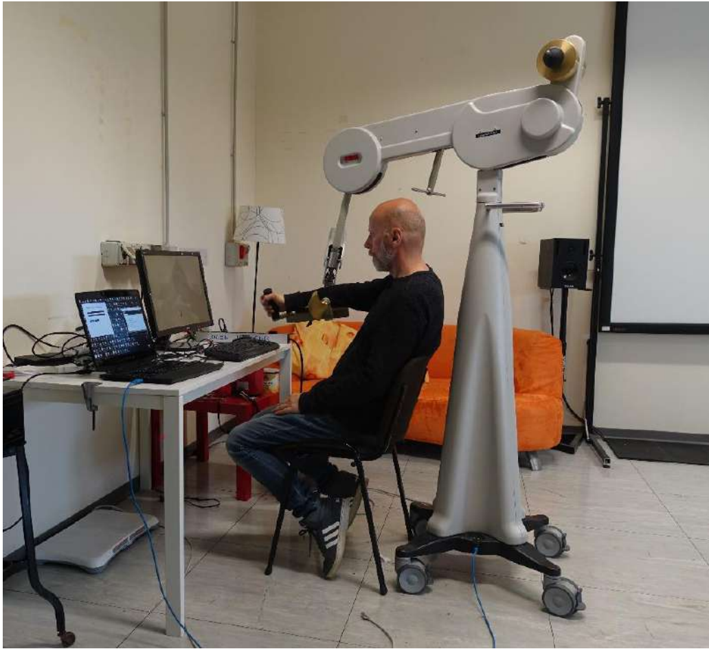
FIGURE 9. Side view of the system, with operator monitor (laptop) and larger display monitor for the subject.
