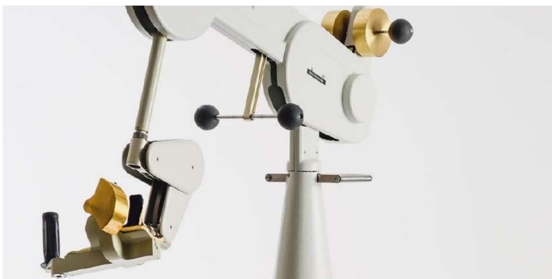
FIGURE 7. The body of the passive robotic arm called Track-Hold.
