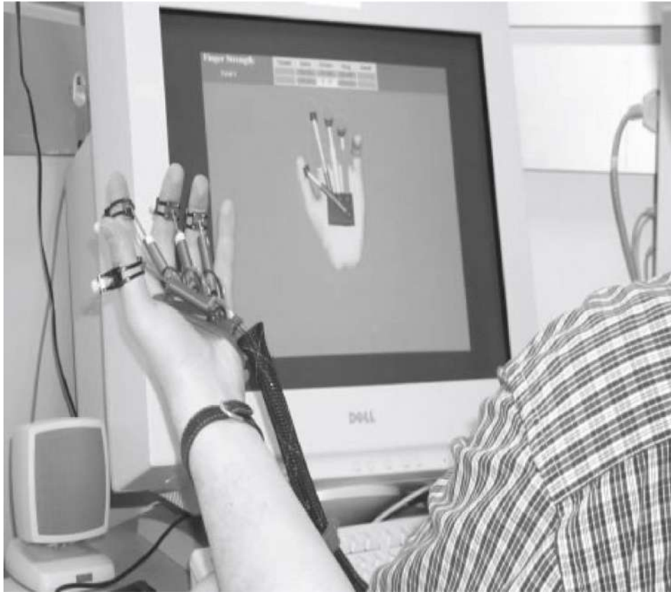
FIGURE 6. Rutgers Master II force-feedback glove.
